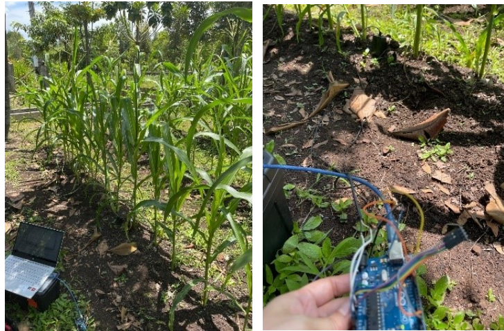
Figure 5. pH and humidity data collection in the sugarcane field
